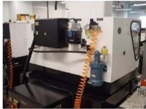
(b) Pneumatic system of an automatic machine
